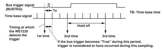
In addition, the WE7235 can output a bus trigger signal upon detecting a trigger within the module, and receive the results of the AND/OR computation on the bus to trigger the actual trigger operation.
